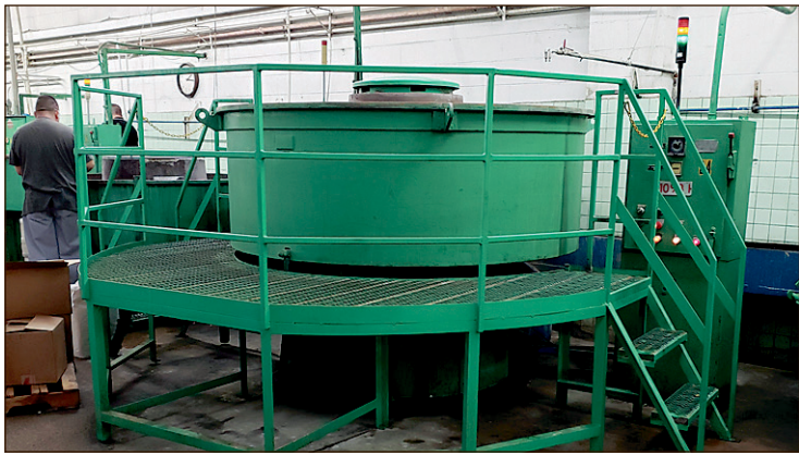
A vibratory tumbling machine on the shop floor at KVF Company processes helicopter gears. (Photo by Melanie Kalmar)
